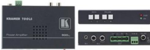
The 900xl is a high-performance power amplifier for line level stereo audio signals. The unit accepts unbalanced audio signals on either of two RCA or 3.5mm connectors and delivers a speaker output of 10 watts RMS per channel into a 4Ω load
